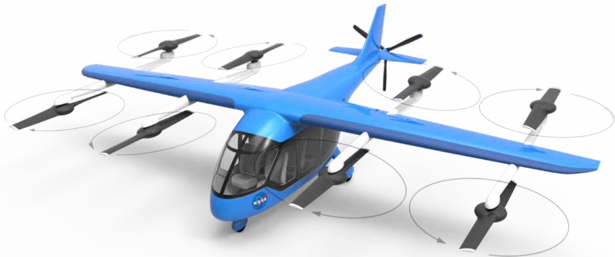
Figure 1.2 CAD Rendering of the Lift+Cruise Concept Reference Vehicle
